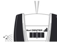
In cases of deeper studs (thicker walls), when the center of the stud is located only two bars will show on the Signal Strength Indicator and only the SpotLite Pointing System will all illuminate. If you still cannot locate a stud, try STUD DEEPSCAN mode. In STUD DEEPSCAN mode, the Stud icon will continuously flash.
